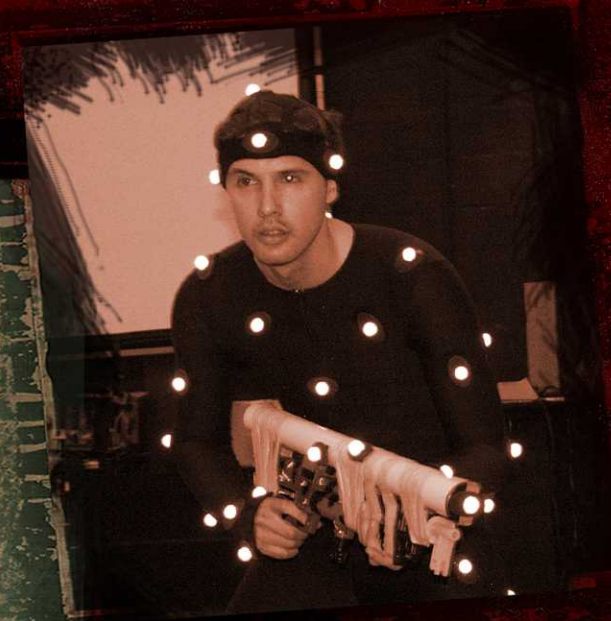
MOTION AND FACIAL CAPTURE WERE USED TO ENSURE REALISTIC MOTION OF THE CHARACTERS
